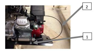
3) Using the motor's existing throttle linkage hardware, attach the throttle cable. The cable should be connected in two positions. One to secures/stabilizes the cable, and another to control the throttle.
