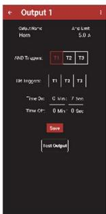
**Output Configuration** The configuration page is used to configure output settings including: output name, amperage limit, time on, time off, trigger logic (and/or). Tap “Save” to save the configuration to the Amplink. Tapping the back button will discard changes and exit the configuration screen.
