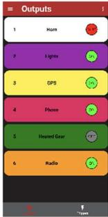
**Output** The output page allows for monitoring the current state of the outputs of Amplink device. The colored bars match the wire color of the corresponding output on Amplink PDM. The output status is indicated by either a green dot for ON, red dot for FAULT, or gray dot for OFF. By tapping an output, the Output Configuration page will appear.
